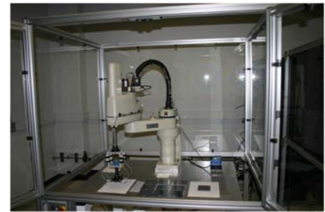
Figure 2. 4-axis wafer handling robot equipped with sensors.
